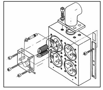
The flow meter is designed to pass a small flow even if the gears are prevented from turning due to solid particles contained in the oil. This prevents complete starvation of oil to bearings etc.
