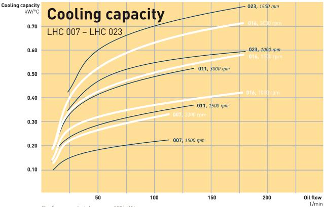
Cooling capacity tolerance  $\pm$  10% kW.
