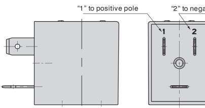
Coil terminal with DC specification has polar indicator lights, thus when wiring, please notice positive and negative poles, "1" shall be connected to positive pole, "2" to negative pole. If the poles are connected incorrectly, the indicator lights will not light up but the valve will still actuate.
