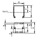
Provides secure wall mounting for individual Excelon products\*
