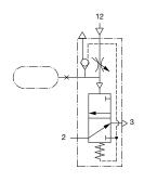
Model Number: **BM/1430**Port for additional reservoir should remain plugged when not used.
