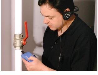
AccuTrak® VPE represents the state-of-the-art in ultrasonic technology for leak detection and preventative maintenance, and incorporates several of the most recent patents in the field. AccuTrak® is extremely sensitive to ultrasonic sound of turbulence and friction that is associated with costly equipment faults. Using a technique called "heterodyning", AccuTrak® translates
